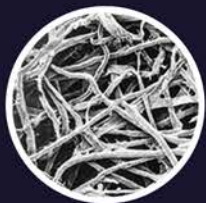
Clean fuel filter
